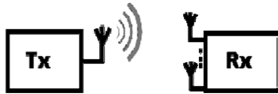
Fig. 5.6 SIMO (Single Input Multiple Output)
