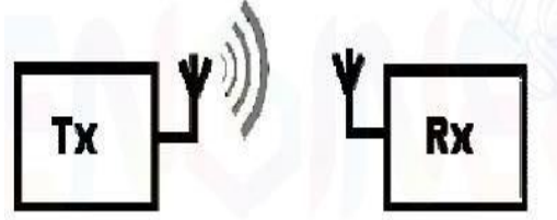
Fig. 5.5 SISO (Single Input Single Output)
