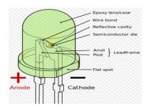
When the diode is forward biased, then the electrons & holes are moving fast across the junction and they are combining constantly, removing one another out. Soon after the electrons are moving from the n-type to the p-type silicon, it combines with the holes, then it disappears. Hence it makes the complete atom & more stable and it gives the little burst of energy in the form of a tiny packet or photon of light.
