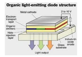
A typical OLED is composed of a layer of organic materials situated between two electrodes, the anode and cathode, all deposited on a substrate.
