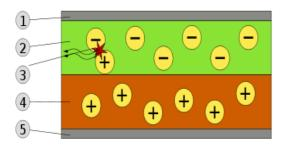
During operation, a voltage is applied across the OLED such that the anode is positive with respect to the cathode.
