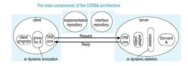
CORBA provides for both static and dynamic invocations. Static invocations are used when the remote interface of the CORBA object is known at compile time, enabling client stubs and server skeletons to be used. If the remote interface is not known at compile time, dynamic invocation must be used. Most programmers prefer to use static invocation because it provides a more natural programming model.
