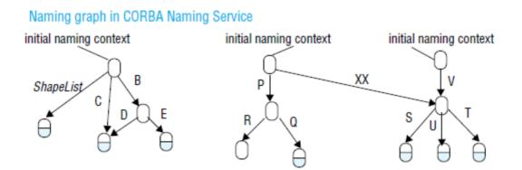
a *naming context* is the scope within which a set of names applies – each of the names within a context must be unique. A name can be associated with either an object reference for a CORBA object in an application or with another context in the naming service.
