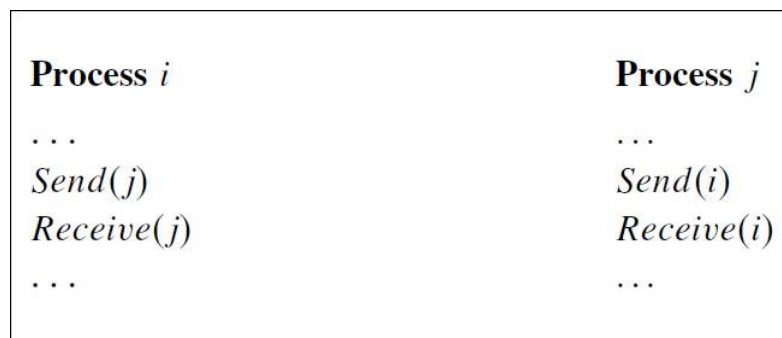
Figure A communication program for an asynchronous system deadlocks when using synchronous primitives.
